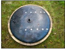
After the lift, a number of bolts were fitted to make to the structure secure and further work will take place on the smokebox as the weather allows. Other jobs completed this month include putting together a wooden former which will be used to make a pattern for the smokebox ring and drawing up detailed plans for the smokebox door straps and hinges.
